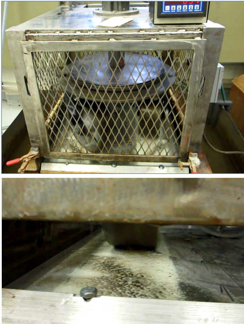
Figure 4.6 Accelerated wearing of samples from test deck.
