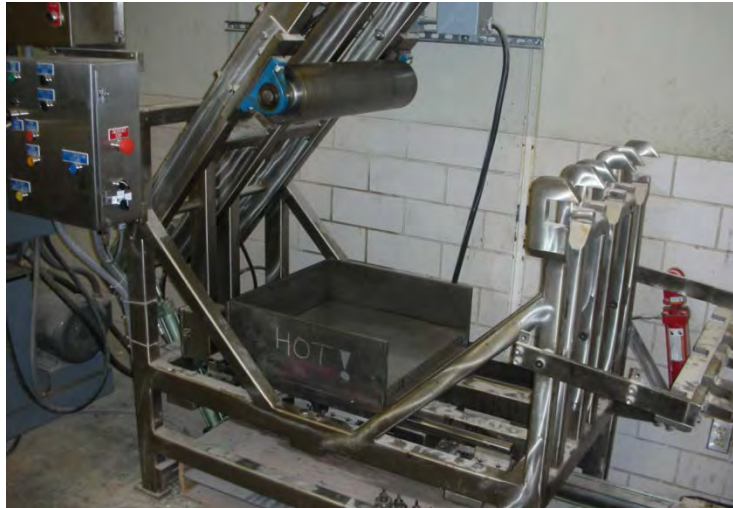
Figure 4.1 Linear kneading compactor for preparing asphalt slabs.
