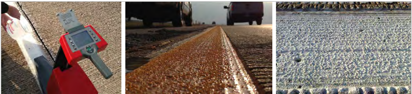
Figure 3.2 Taking a retroreflectivity (recovery, left) reading on I-55 along with marking presence images for the yellow edge line (center) and white edge line (right).
