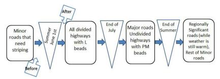
MoDOT striping plan starting in 2015 (with the introduction of a new type of beads for divided highways that require higher drying temperatures)
