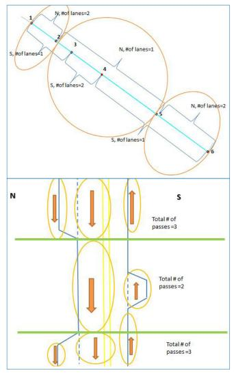
Example of "difficult" segment for which number of passes and end/start points are different (top) and how the segment looks with the different number of passes for striping operations (bottom)
