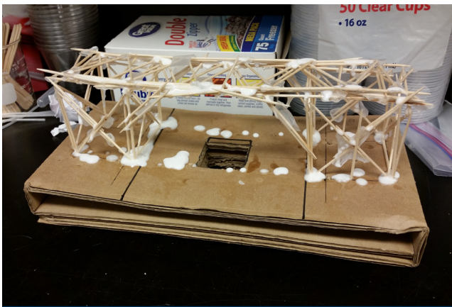
Test bridges were made out of toothpicks and Elmer's school glue
